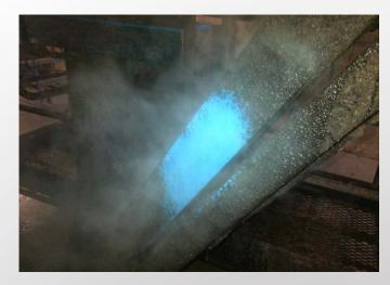
A successful field trial was commissioned and completed by a client seeking to reduce or eliminate the cost of having their equipment (seen above – section of a boom) sand-blasted by a third party to remove encrusted bitumen after use in the field. The results of this trial lead the client to complete cleaning and degreasing of their field equipment internally at a substantially lower cost.
