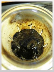
Laboratory demonstration of the surface cleaning capacity of CITRIKLEEN® CR34 against a competitor's product. An excessive weight of diluted bitumen was exposed to equal volumes of each product, pulled out and rinsed at intervals before completely dissolved. Each time, CITRIKLEEN® CR34 (far left) dissolved more material and provided cleaner rinsing of all surfaces.
